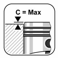
The measurement must be performed for all pistons. The piston with the highest projection is used to determine the matching cylinder head gasket.
