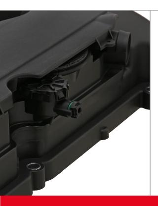
In the case of vehicle models that have been specially manufactured for the Korean or American market, the open valve plug has to be mounted instead of the red sealing plug. Can be seen in the image on the left.
