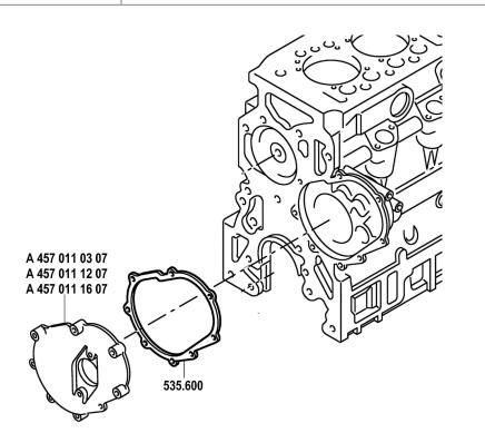
In order to improve seal performance between the camshaft sprocket cover and the engine block, a new Metaloseal<sup>®</sup> has been developed. It replaces the sealing compound that was prviously used for this joint.
